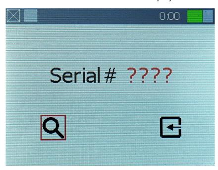
If the "magnifying glass" field is activated, the connection display blinks in the upper left of the status bar as a blue square. After the search operation is completed, the square is lit up blue continuously. On the screen, the last 3 or 4 numerals of the serial number are now displayed in red behind the designation "Serial" of the located RedDot target.
